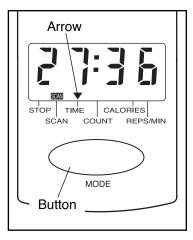
until an arrow points to the name of the desired mode. Make sure that the Scan mode is not selected.
